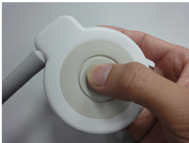
Figure 7-5 Testing a TOCO Transducer
