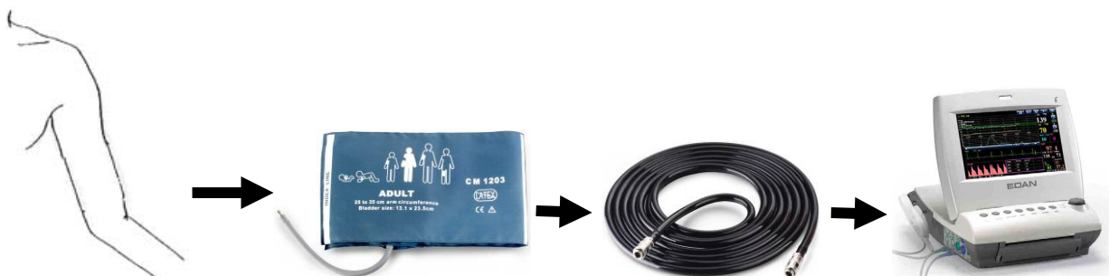
Figure 9-5 Connection for NIBP Measurement
