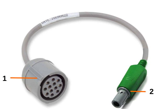
Figure 3-14 IUP Connecting Cable
