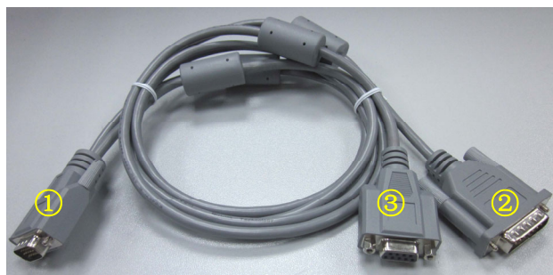
Figure A7-2 Y-shape Signal Cable
